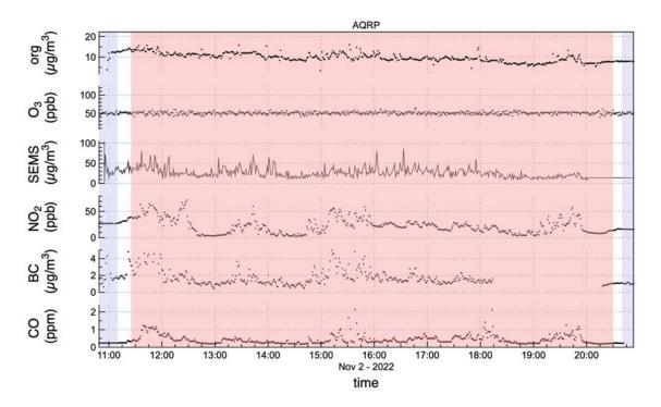
**Figure 22-020-6**. Time series data of major instruments during the fall deployment in Houston (Nov. 2<sup>nd</sup> as an example)
