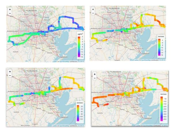
**Figure 22-020-7**. Concentration of aerosol mass concentration and three major VCPs sampled on November 2<sup>nd</sup> in Houston. The upper left is total organic aerosol mass loading. The upper right plot is texanol. The lower left and lower right plots are D5-siloxane and monoterpenes.
