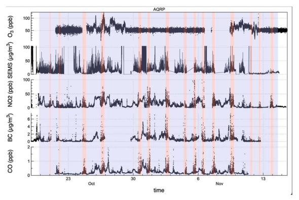
**Figure 22-020-3**. Aerosol Mass, Ozone, CO, NO<sub>2</sub>, and black carbon measurement during the whole deployment. The purple shaded areas were when vehicles are parked, and the orange shaded areas were when instruments are deployed in motion.
