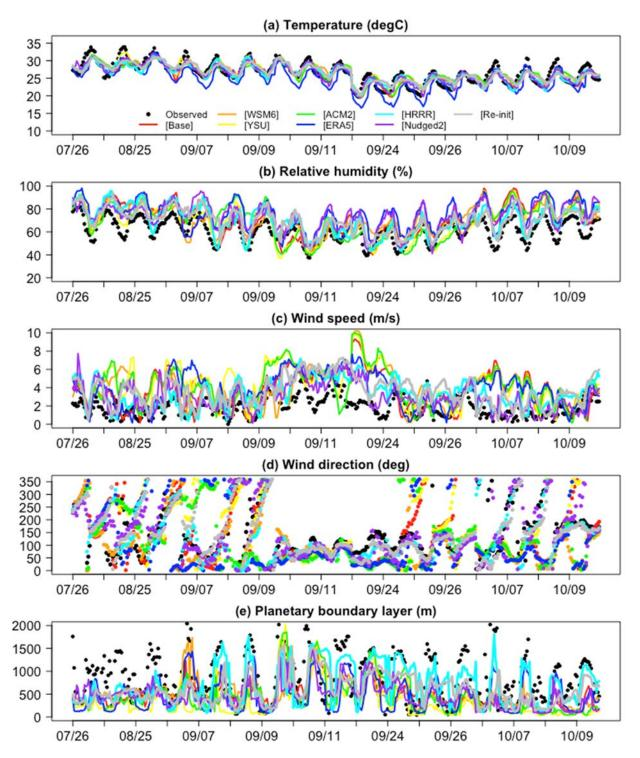
**Figure 22-008-4.** Time series of (a) air temperature, (b) relative humidity, (c) wind speed, (d) wind direction and (e) boundary layer height between 1-min boat observations and WRF model
