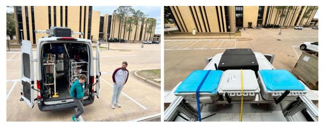
Figure 22-020-9. Exterior and roof top (with three air sensors) view of the mobile laboratory
