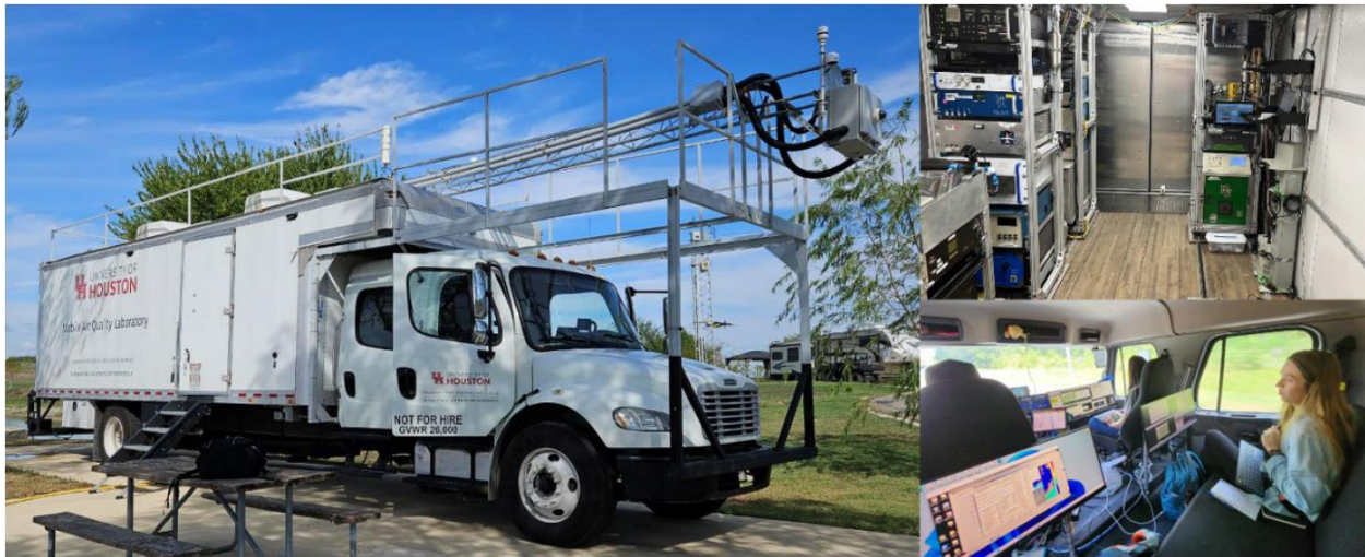
Figure 1. Photos of MAQL3. The upper right photo shows an example of instruments installed in the rear lab space and the lower right image shows an example of the operator stations in the cab.
