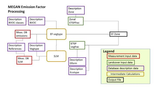
Figure 1. Schematic of MEGAN emission factor processing.
