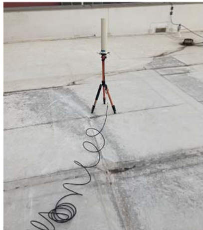
Figure 20-004-1: The Harsh/Synergetics 14A-N omnidirectional antenna mounted on a tripod.
