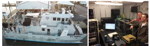
Figure 1. The proposed measurement vessel (left), the Research Vessel Trident, owned and operated by Texas A&M University out of Galveston. This vessel's laboratory space (right) is used to house measurement instrumentation.
