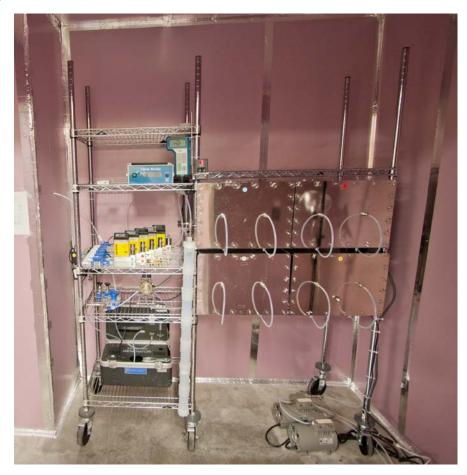
**Figure 1.** Experimental system for the ozone deposition experiments.
