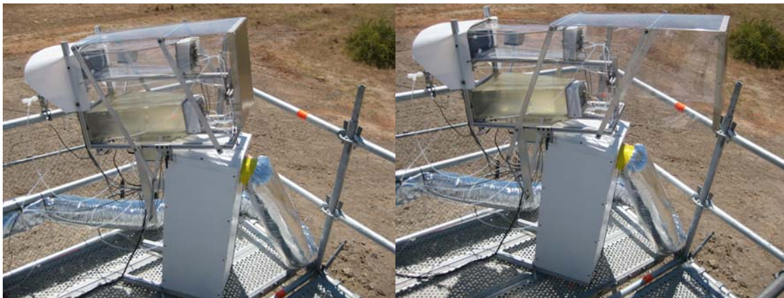
Figure 2. MOPS zeroing cover closed (left) and MOPS zeroing cover in the open position (right). The cycling of this UV absorbing cover every 10 minutes has proven to be the best way to achieve an effective instrument “zero”.
